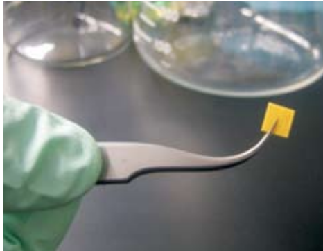
The PoLi implant that provides sustained release of the anti-cancer agent, paclitaxel.
